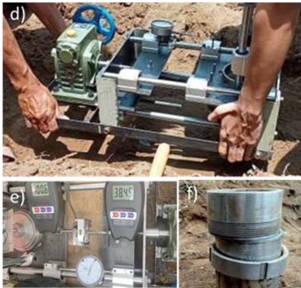
Figure 4. Testing step: a). placing the sampler tube, b). inserting the tube into the soil, c). excavating soil out of the tube, d). setting device, e). setting all the measurement tools and start testing and f). sheared sample after the completed test
