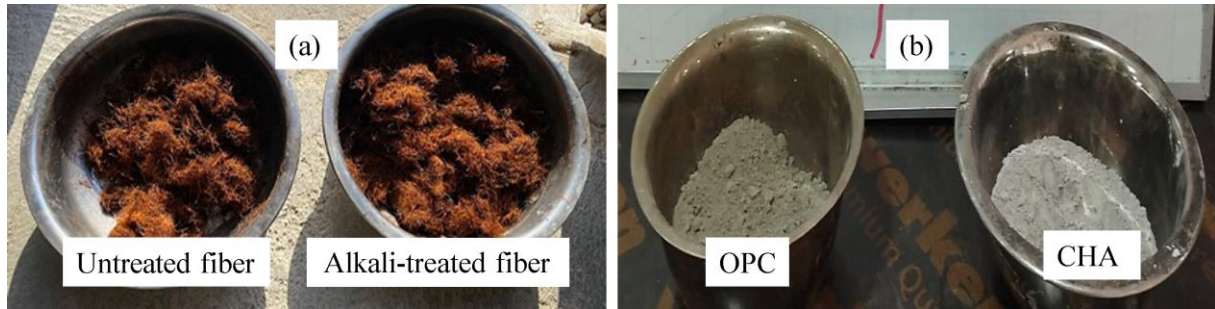
Notes: (a) Fibers before and after alkaline treatment; (b) OPC vs. CHA; from left to right
