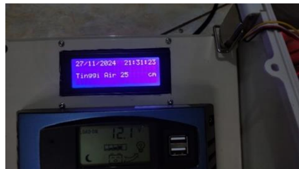
Figure 5. Setting the Accuracy Test of the Water Level Sensor
