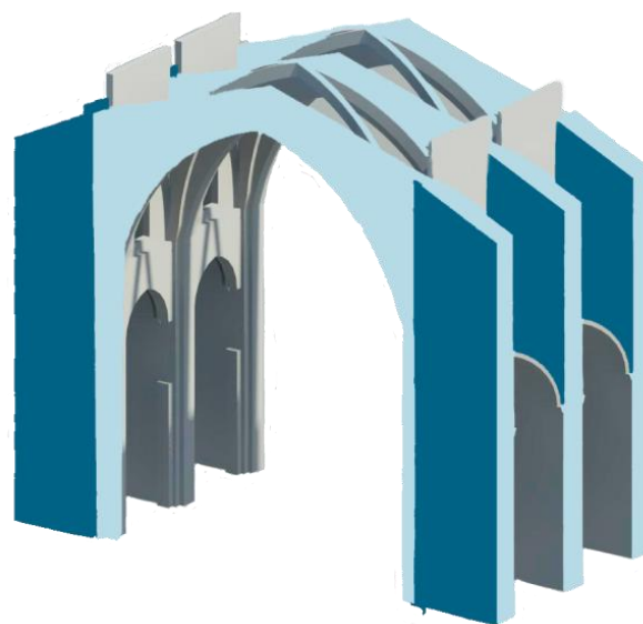
Figure 5. Structural system of Los Santos Juanes
