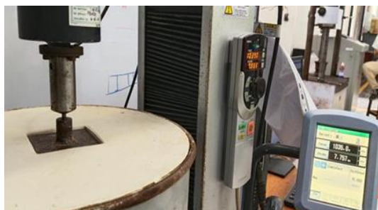
Figure 7. Soil shear failure test ( q_{ult} ) on soft clay soil
