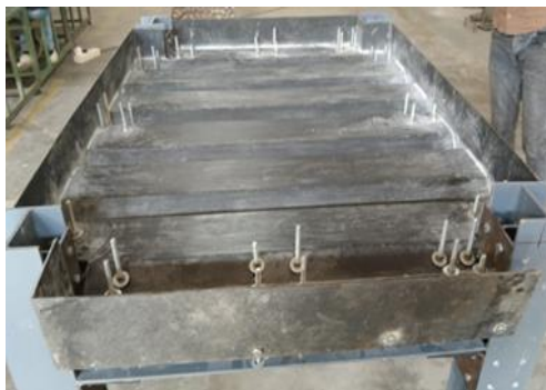
Figure 3. Fabricated GFRP sheet profile
