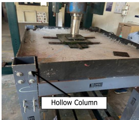
Figure 10. Test set-up of hollow frame
