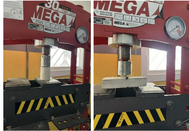
Figure 3. Compression and flexural tests performed with a hydraulic press
