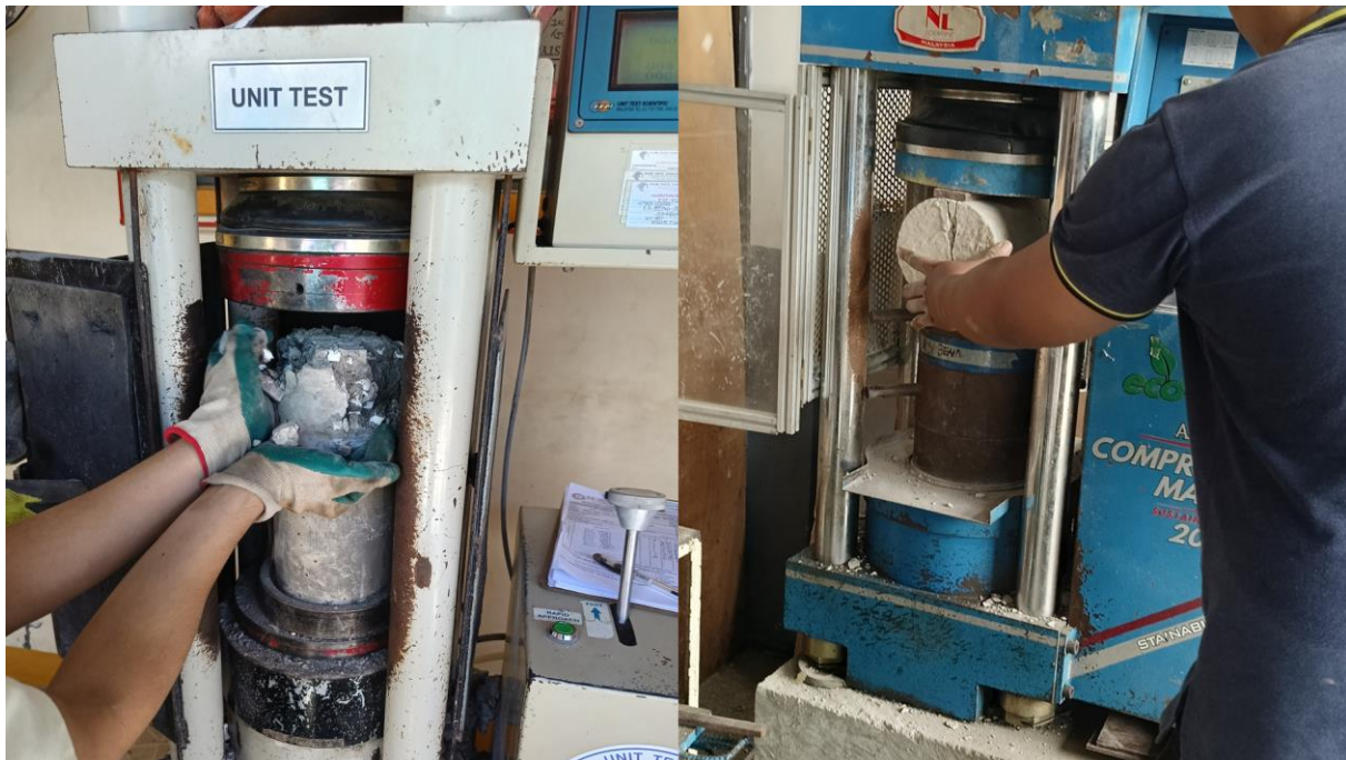
Figure 1. Testing setup for compressive (left) and split tensile strength (right) showing specimen positioning, applied load direction, and measurement configuration for EPS-based concrete specimens
