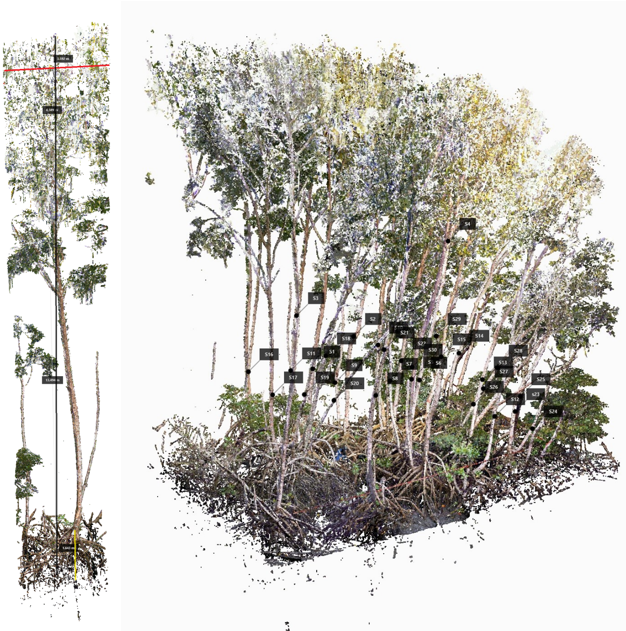
Figure 9. (Left) Example of a mangrove tree quantification from TLS point cloud. (Right) Overview of 30 individual mangrove trees identified within a 10 \times 10 \text{ m}^2 domain.
