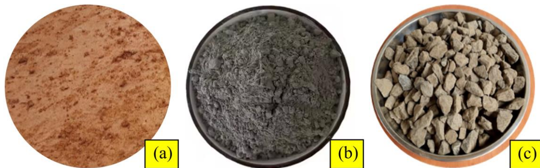
Figure 1. (a) Existing Soil (OPC), (b) Ordinary Portland Cement (OPC), (c) Coarse Aggregate
