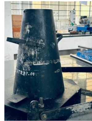
Figure 3. Slump cone apparatus used to study the workability of the mixes
