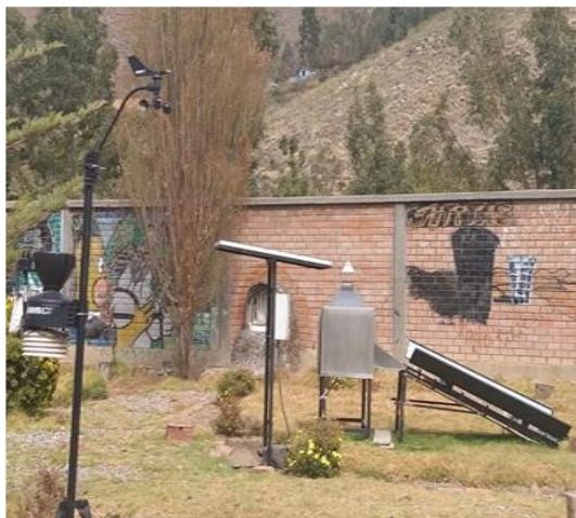
Figure 3. Weather station and automated solar drying system
