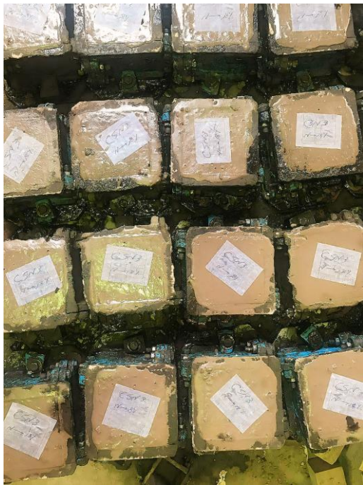
Figure 4. Specimens after casting and curing
