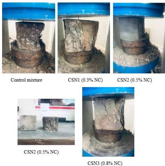
Figure 16. Mechanisms of failure of the cubes
