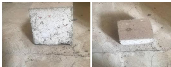
Figure 17. Shape of cube surface after exposure to 700 °C for 2 hours (cooling in furnace)
