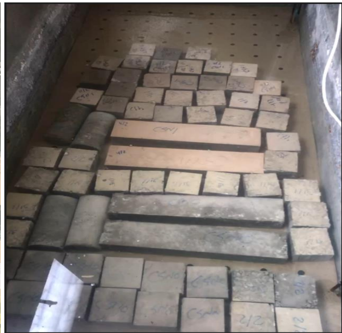
Figure 5. Curing of the specimens in water
