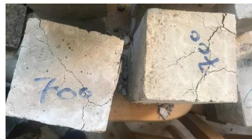
Figure 18. Shape of cube surface after exposure to 700 °C for 2 hours (cooling in air)
