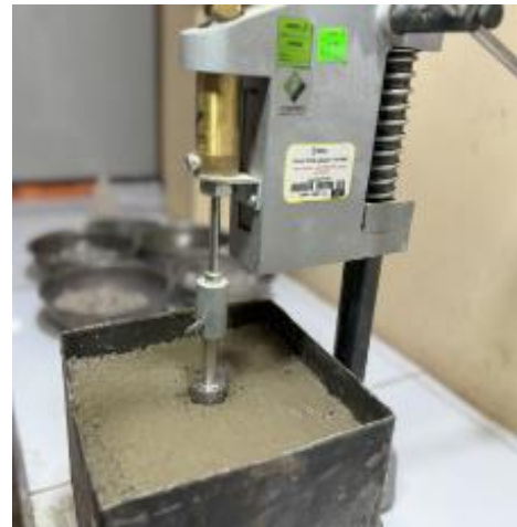
Figure 5. Setting Time Determination using the Vicat Needle
