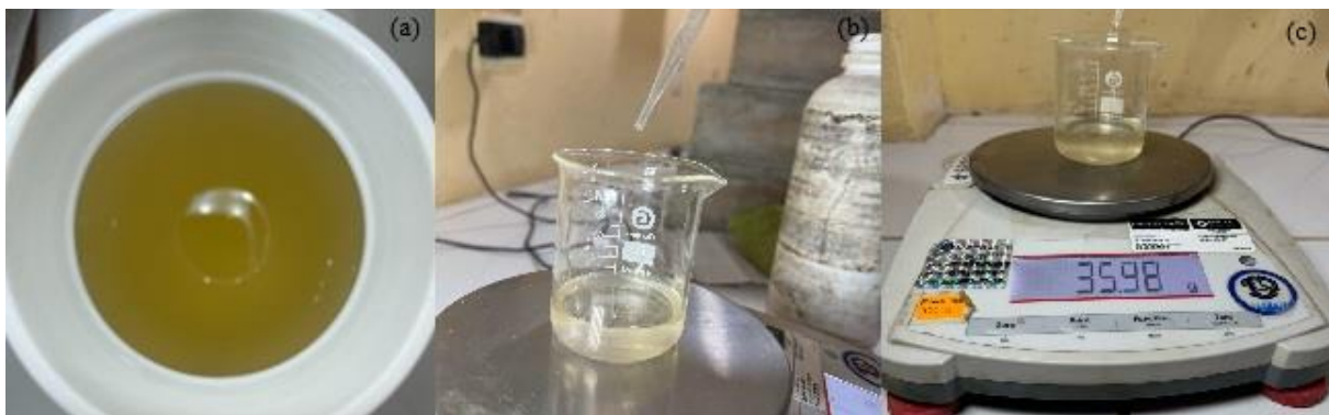
Figure 3. Steps in the admixture dosage determination process: (a) initial solution, (b) dilution, and (c) weighing
