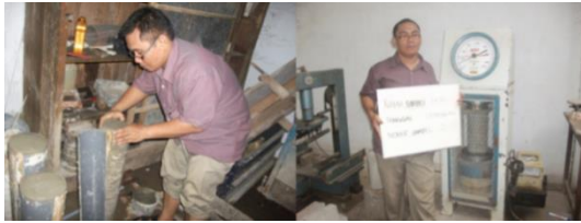
Figure 6. Release of molds and concrete quality testing
