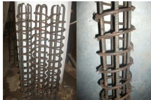
Figure 5. Configuration of concrete column reinforcement
