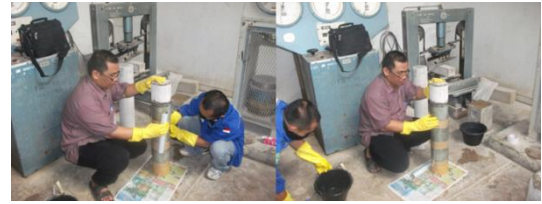
Figure 8. The process of wrapping the full GFRP layer
