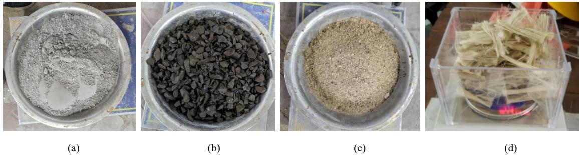
Figure 1. Materials used in the study: (a) cement, (b) coarse aggregates (stone chips), (c) Fine aggregates and (d) 25 mm jute fibers
