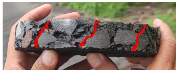
Figure 1. Surface water flow through interconnected gaps and partly through vertically connected cavities
