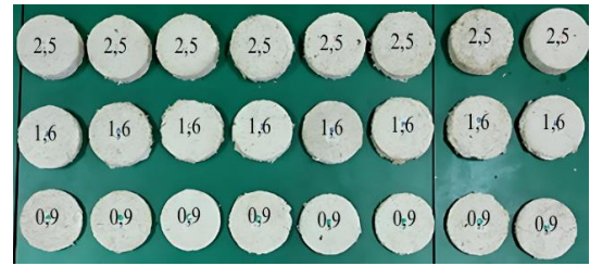
Figure 1. 10 cm circular test sample with 3 thicknesses (0.9; 1.6; 2.5 cm) a total of 24 pieces
