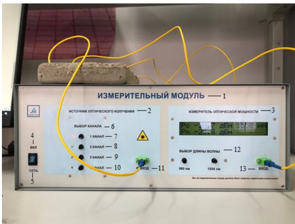
Note: 1 – measuring module; 2 – the source of optical radiation; 3 – optical power meter; 4 – on; 5 – network; 6 – channel selection; 7 – channel 1; 8 – channel 2; 9 – channel 3; 10 – channel 4; 11 – output; 12 – wavelength selection; 13 – input.
