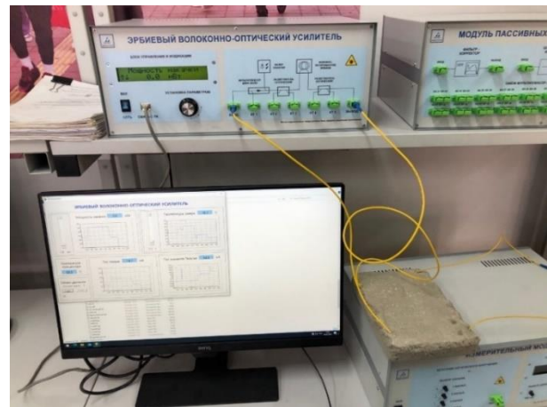
Figure 6. Temperature determination of optical sensors based on concrete
