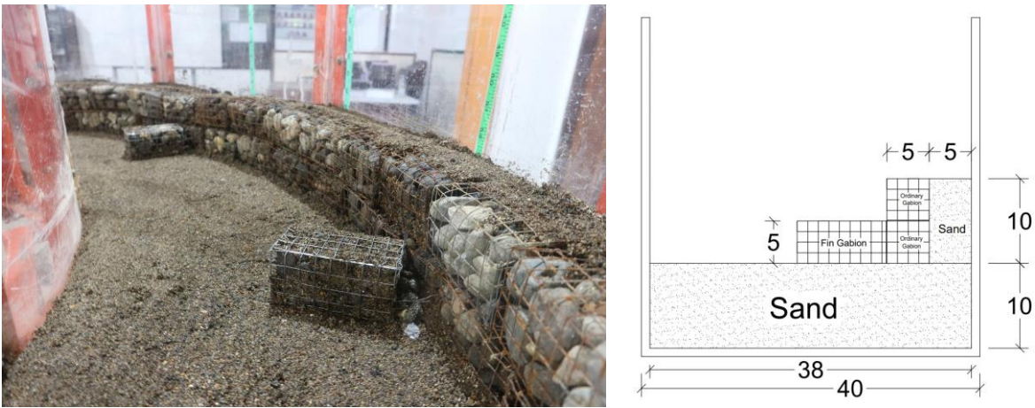
Figure 13. Setup-5 before simulation (photo and sketch viewed from upstream)
