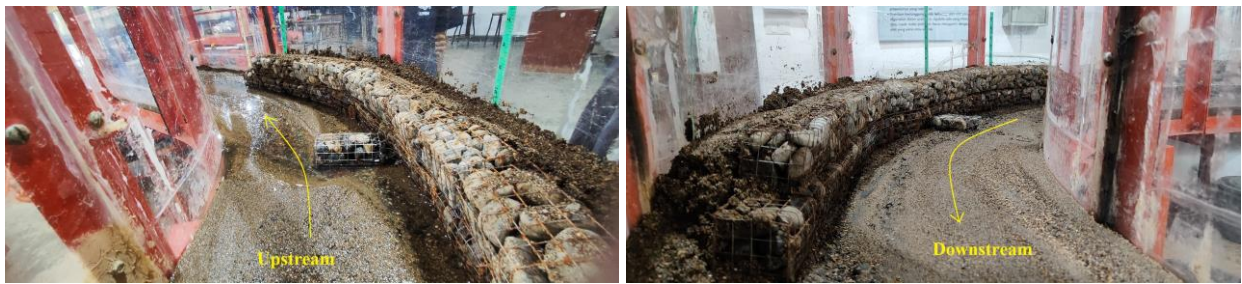
Figure 7. Post-simulation (Setup 2) condition of the regular gabions and fin gabion at the lower part of the bend, viewed from upstream and downstream
