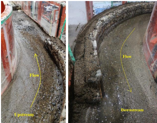
Figure 5. Flume bed topography after the initial simulation (Setup 1), showing the development of a sediment deposit near the inner bend and erosion near the outer bend in all three sections of the bend
