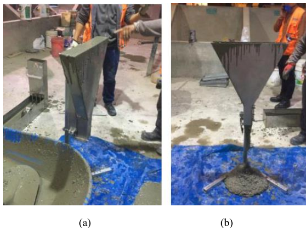
Figure 5. Box V. (a) Concrete poured and screeded in box V, (b) Exit of concrete through box V
