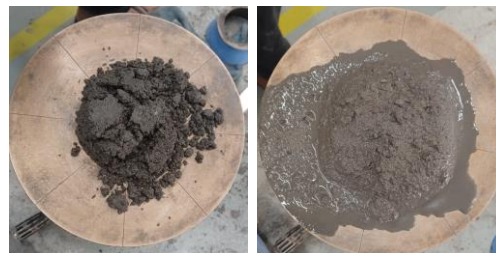
Figure 20. Spread of Flow Table Test for Mortar Mixes incorporating CBA at replacement levels of (a) 0% and (b) 75%
