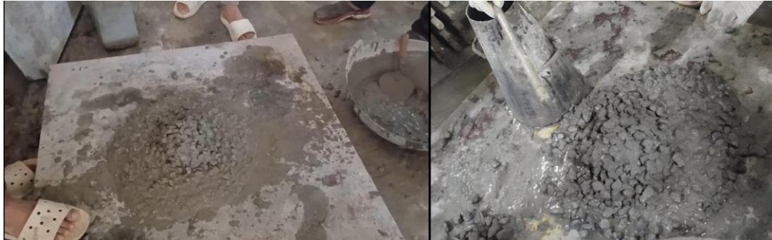
Figure 10. Slump Patterns of (a) CBA0 and (b) CBA75
