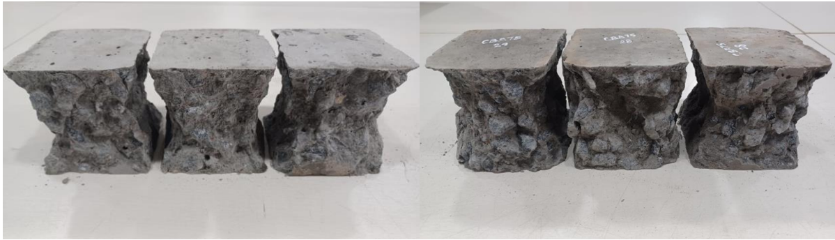
Figure 13. Failure Pattern of (a) CBA0 and (b) CBA75 under compressive stresses
