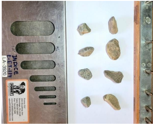
Figure 2. Fractured Particles (Sharp Edges, Rough Surfaces)
