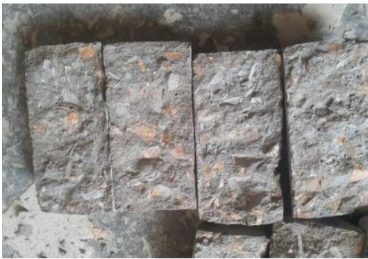
Figure 18. Result of the tensile strength test failure
