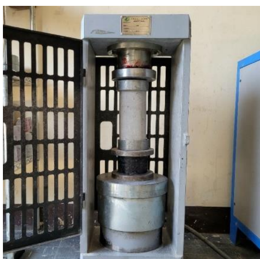
Figure 5. Compressive Strength Test
