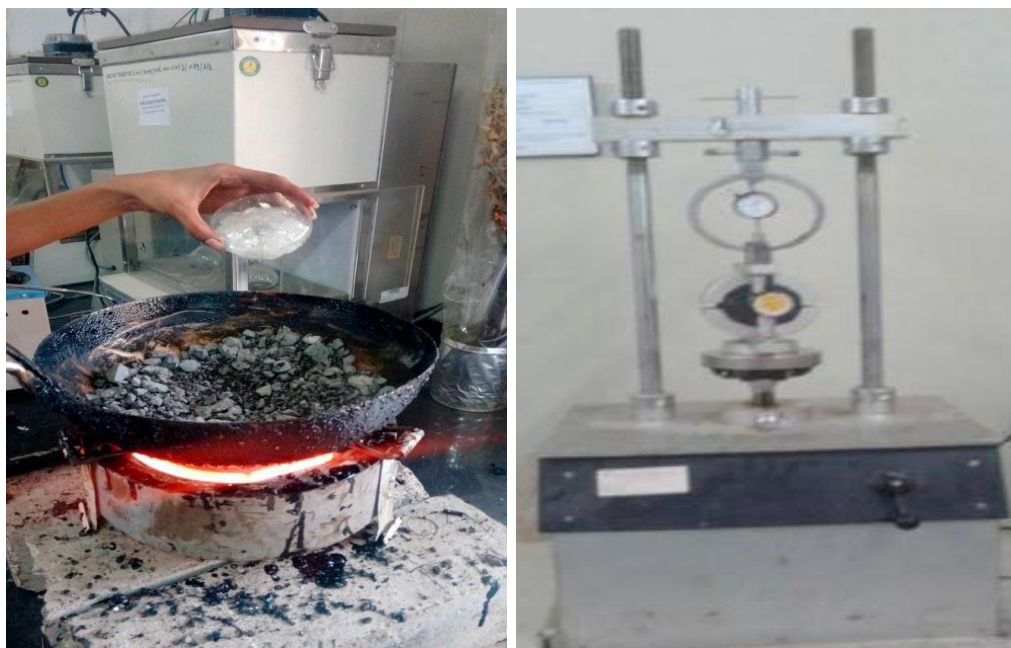
Figure 7. Mixing crushed plastic waste into aggregates and sample arrangement in Marshall test setup [20]
