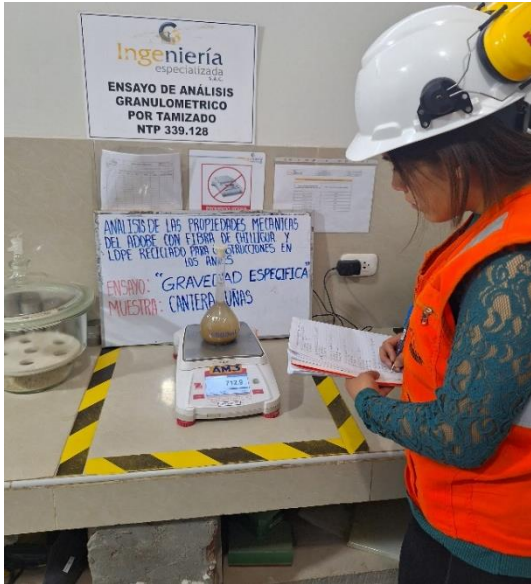
Figure 12. Specific gravity test using the water pycnometer
