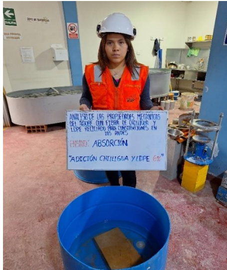
Figure 16. Absorption test of samples 0,1,2,3,4,5,6 % addition of Chillihua and LDPE
