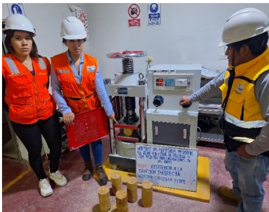
Figure 13. Indirect tensile test on specimens 0, 1, 2, 3, 3, 4, 4, 5 and 6% addition of Chillahua and LDPE
