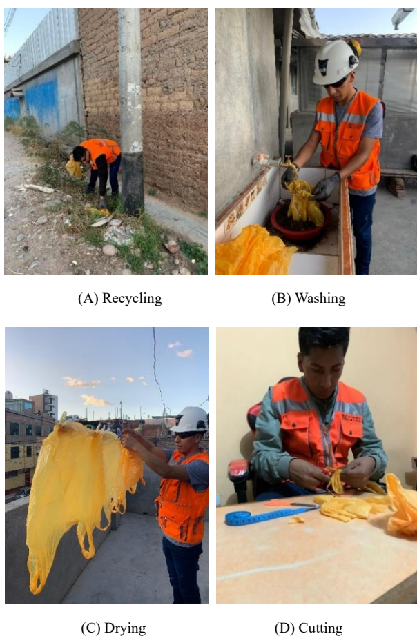
Figure 3. LDPE fibre production process
