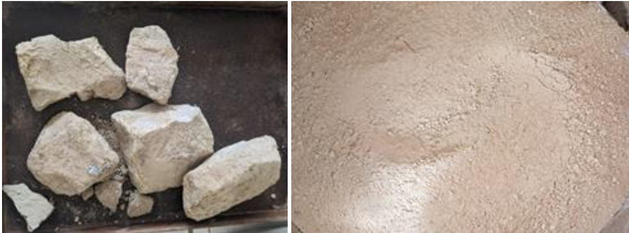
Figure 1. Moroccan Clay used in this study before and after crushing
