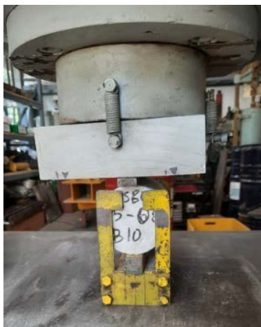
Figure 5. Tensile Test of Cylinder specimens
