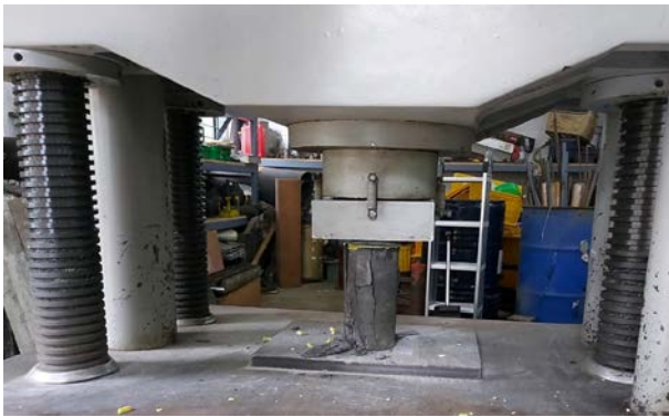
Figure 4. Compressive Strength Test of Cylinder Specimens
