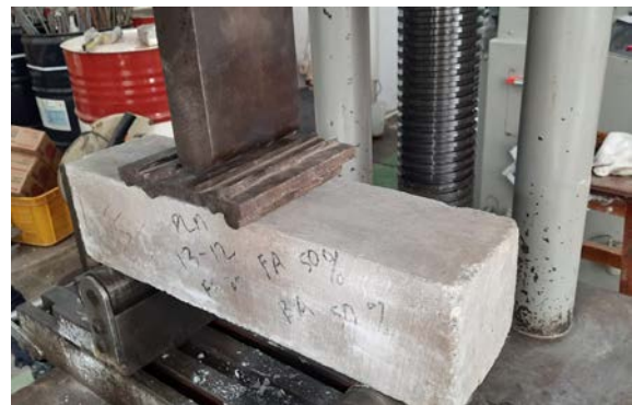
Figure 6. Flexure Test of Beam Specimens
