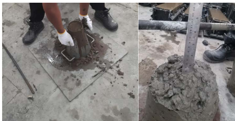
Figure 3. Measurement Process of Slump
