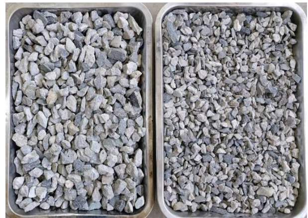
Figure 2. RCA at \frac{1}{2} " (12.5 mm) and 1-1 (9.5 mm) sizes
