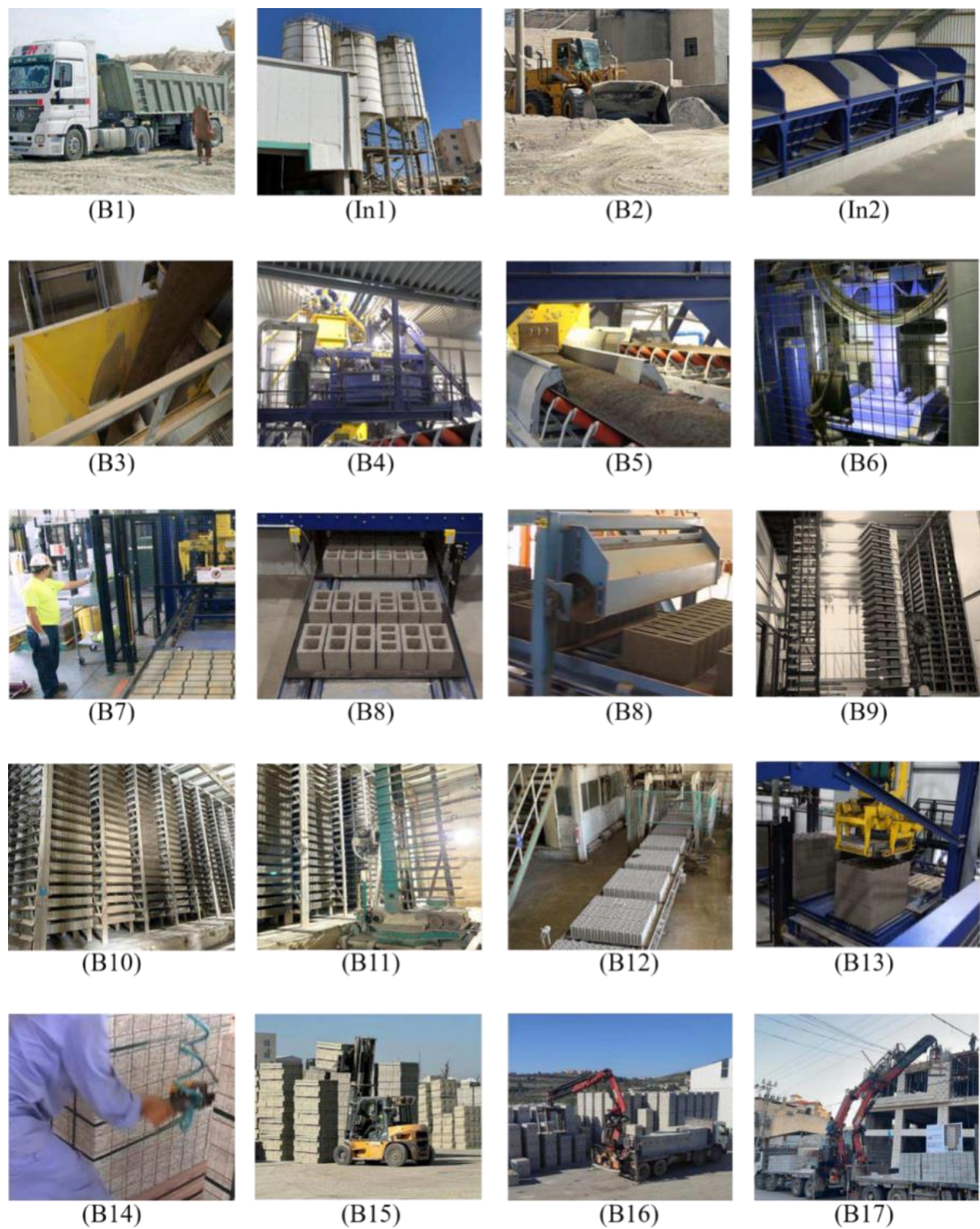
Figure 6. Array of photographs shows full-automatic HCB production from essential materials supply to construction site, refer to table 9
