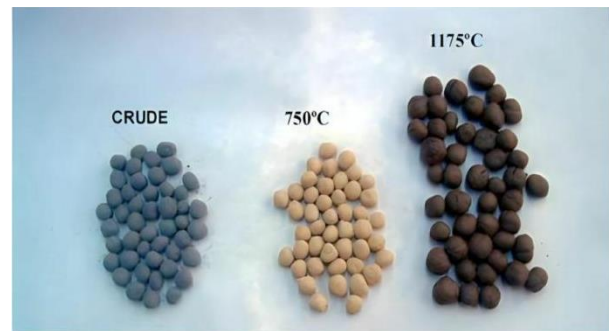
Figure 4. Particles of geopolymers artificial aggregates at different stages of heating [5]
