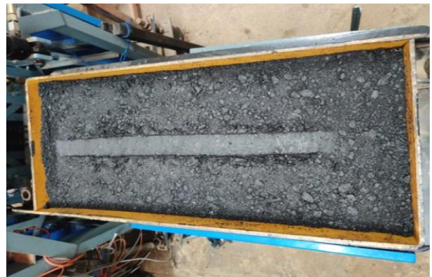
Figure 5. Specimen subjected to Rutting
