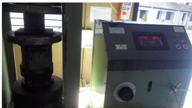
Figure 2. (a) Compression test on cube specimens
