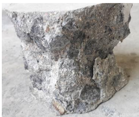
Figure 2. (b) Specimen after compression testing
