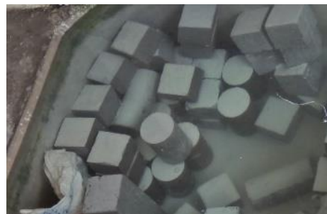
Figure 1. Mixing, Casting and Curing of Moulds
