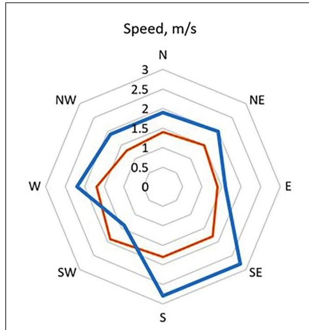
Figure 3. The graph of the wind rose by speed for January and July
