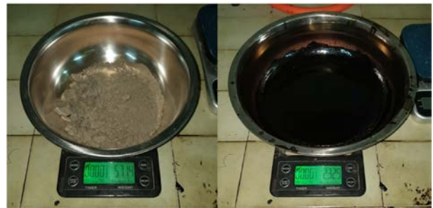
Figure 2. RAP (bitumen and aggregate) extraction
