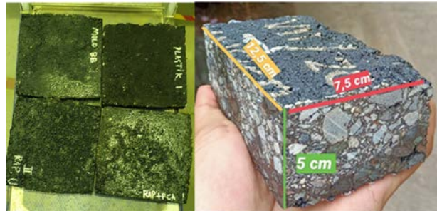
Figure 4. BPT sample printing in the laboratory
