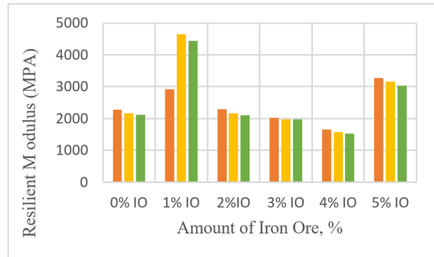
Figure 7. Resilient modulus 25 °C
