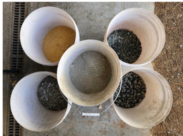
Figure 1. Coarse aggregate, fine aggregate, and fly ash from Bluewater Power Station in Collie, WA (center bucket)
