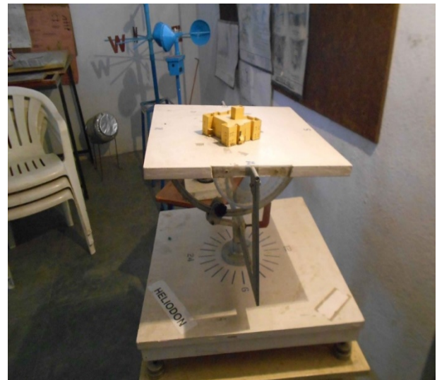
Figure 5. Heliodon shows the Demonstration through Students' Design Models in Climatology Lab.
