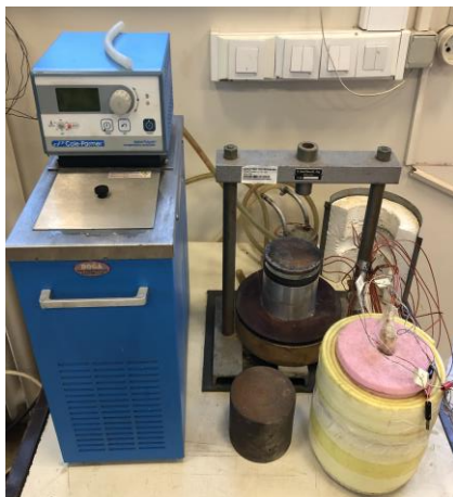
Figure 17. The Experimental Setup, From the Left, Thermostatic Water Bath for Temperature Control, Sample Settlement Part, Istanbul Technical University. Faculty of Mechanical Engineering, Heat Technical Laboratory.
