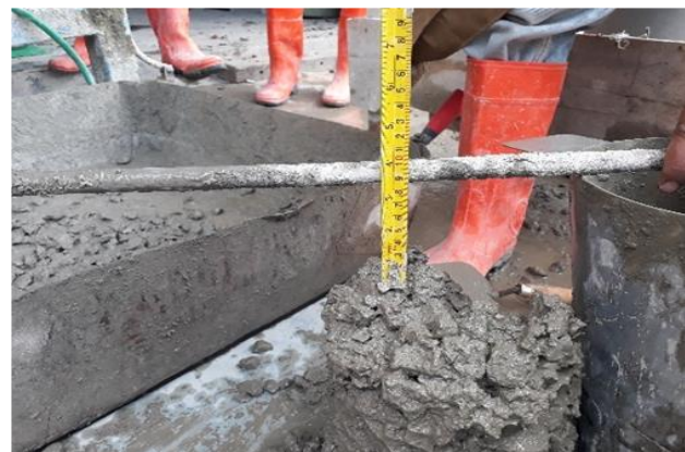
Figure 8. Testing the Slump Test
