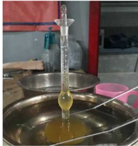
Figure 1. Test the density of cement using a Le Chatelier tube
