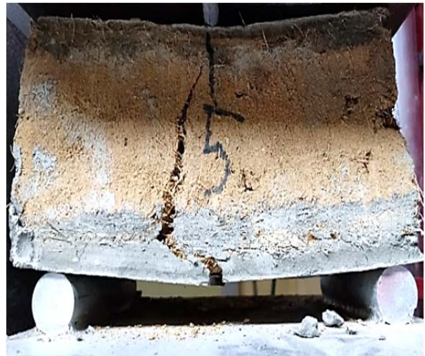
Figure 8. Flexural strength test
