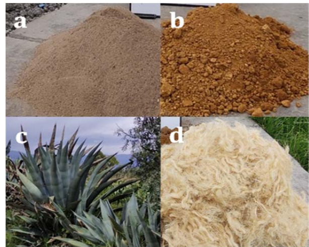
Figure 2. Components of adobe reinforced with Agave americana fiber type "L" (a: sand component, b: clay and silt component, c: Agave fiber in its natural state, d: Agave fiber component)
