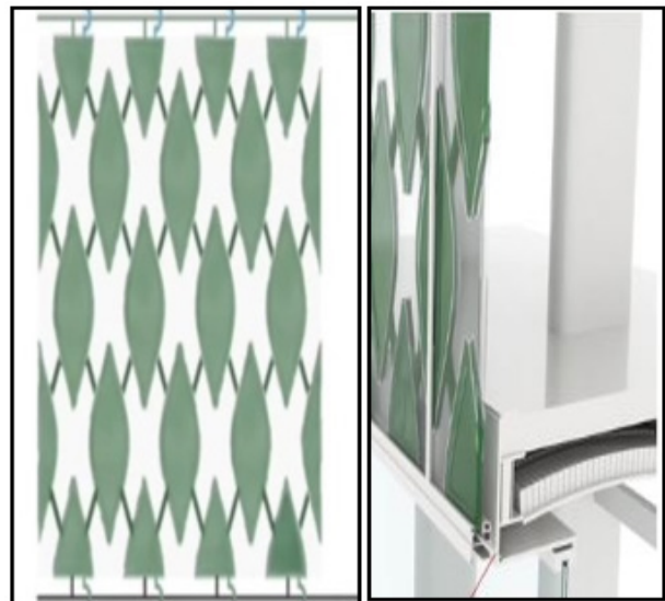
Figure 56. Filling solid parts of opening with algae material [39].
