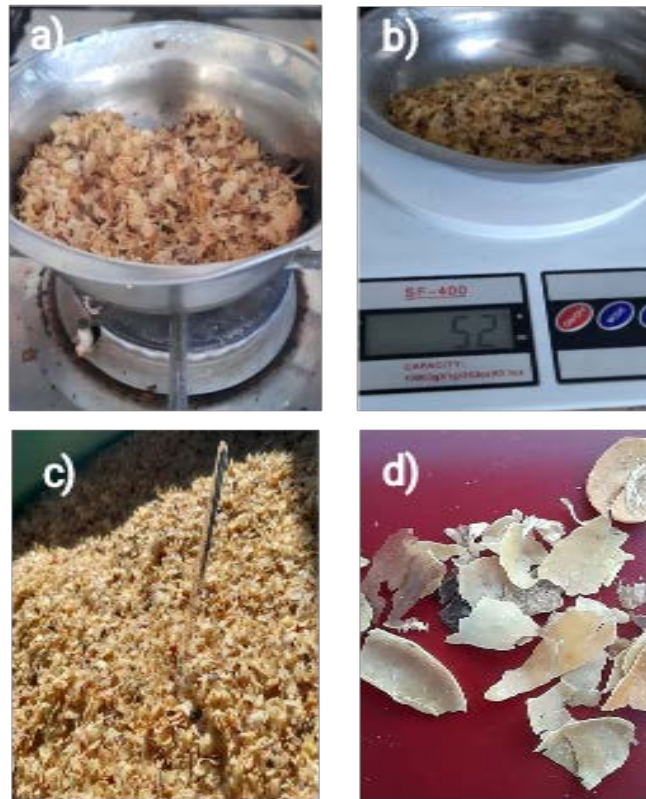
Figure 2. Samples of coffee husk. a) Drying of the sample by the oven method, b) Weight of dry coffee husk + Weight of container, c) Temperature measurement and d) Coffee husk texture in its natural state
