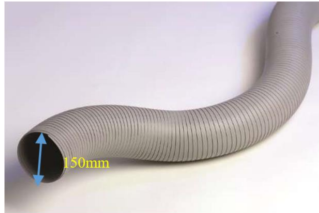
Figure 18. Form of the pipes used
