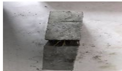
d. weak adhesion of Alfa fibers
