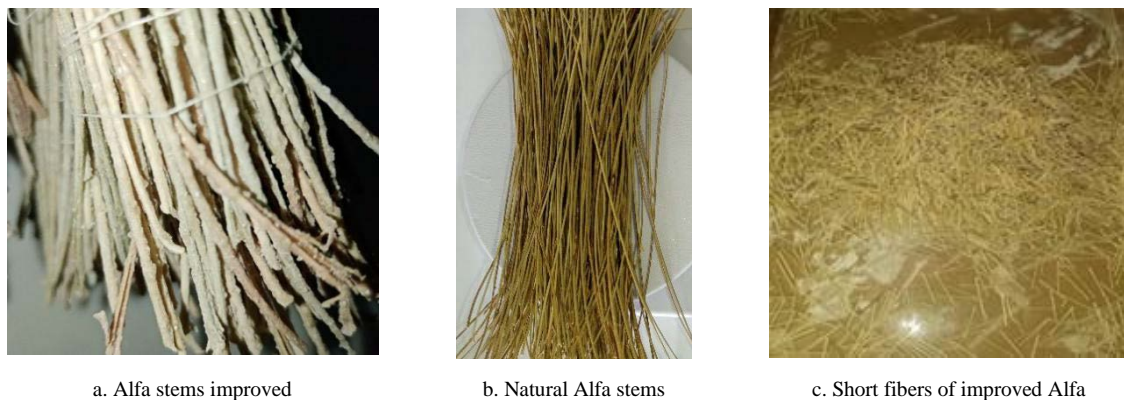
Figure 3. Alfa stems and short fibers improved rough surface
