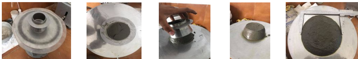
Figure 7. Mortar workability test
