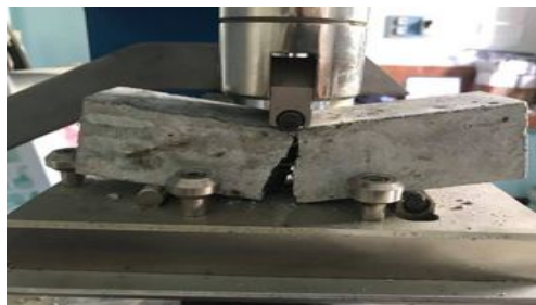
c. control specimen brittle failure
