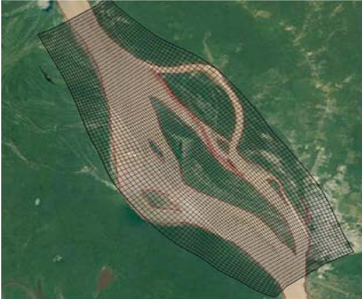
Figure 3. Computational grid for 2D model of the Amazon River
