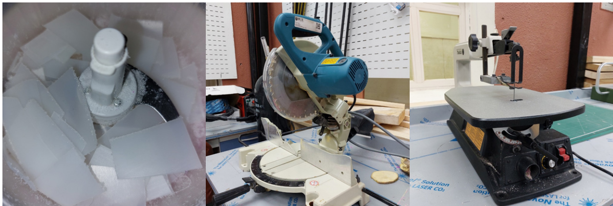
Figure 1. HDPE shredding: (top) knife mill; (middle) pieces cut using the saw;(bottom) saw machine
