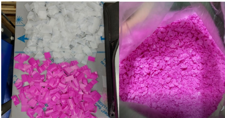
Figure 2. HDPE shredding: (top) Small sized plastic pieces; (bottom) Sand like plastic grains
