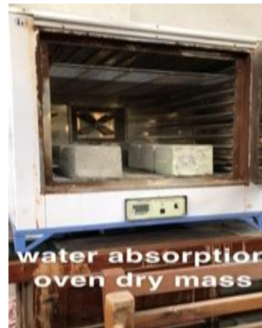
Figure 5. Water Absorption Testing
