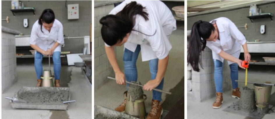
Figure 6A, 6B and 6C. Slump test process with Abrams cone
