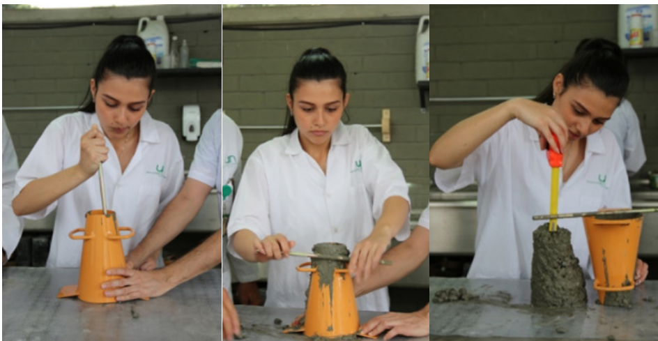
Figure 6A, 6B and 6C. Slump test process with Abrams cone
