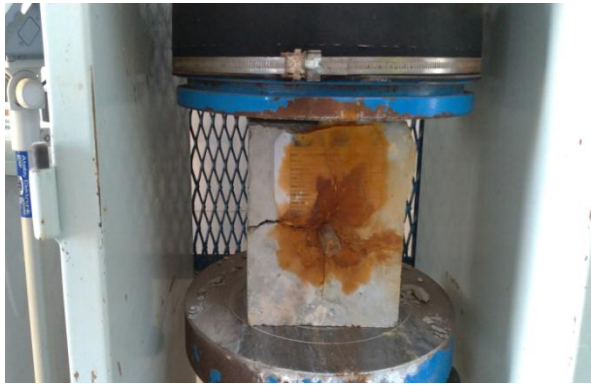
Figure 3. Compressive strength test on concrete
