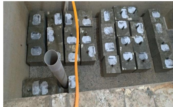
Figure 1. Curing of concrete for 28 days
