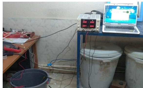
Figure 2. Accelerated corrosion mechanism
