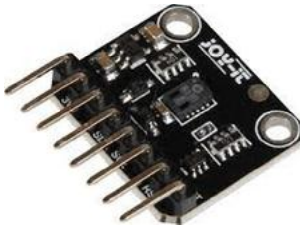
Figure 4. CCS811 Pollutant gas sensor [17]
